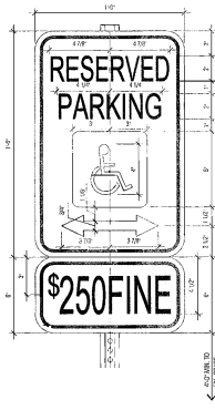
5 H.C. SIGN DETAIL (TYP. FOR 2) SCALE: 3/4" = 1'-0"
